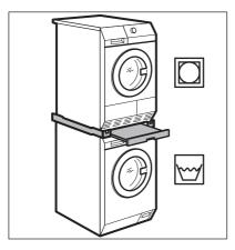
Stacking kit can be used only with the tumble dryers specified in the leaflet. See the leaflet attached. Read carefully the instructions supplied with the accessory.
